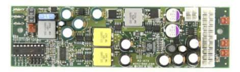
M2-ATX is an intelligent vehicle ATX power supply. Designed to provide power and to control the ON/OFF switch of a motherboard based on ignition status, M2-ATX is a wide input (6-24V) ATX power supply capable of surviving tough engine cranks (down to 5.7V) as well as transient over-voltage situations.
